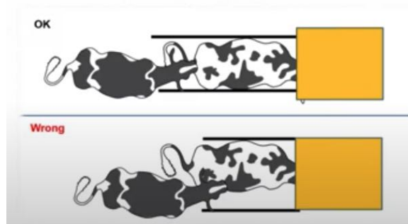
Figure 6) Alleyway Setups to Allow Only One Animal in GreenFeed at a Time
